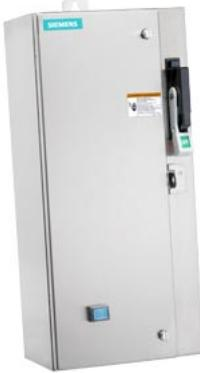
Non-reversing motor starter, Size 0, Three phase full voltage, Solid-state overload relay, OLR amp range 3-12A, 110V 50Hz / 120V 60Hz coil, Combination type, 30A non-fusible disconnect, Encl NEMA type 4X 304 S-Steel, Water/dust tight noncorrosive, Standard width enclosure
