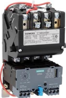
Non-reversing motor starter Size 1 Single phase full voltage Solid-state overload relay OLRelay amp range 5.5-22A 110-120/220-240VAC 60HZ coil Combination type No enclosure
