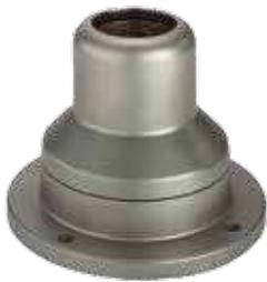
Swivel Base for mounting to machine or floor. Turns through 340 degrees with rotation stop. Preset torque. Maintenance-free bearings. Type 304 polished stainless steel finish. Includes gaskets. Base-mounting fasteners not provided.
