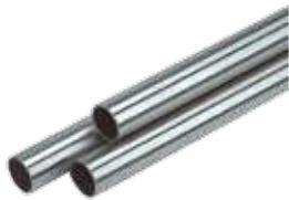
Straight Tubing has an outer diameter of 48.3 mm (1.90 in.) and is made from 3.6-mm wall thickness Type 304 polished stainless steel.
