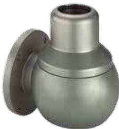
Wall Joint with vertical socket for mounting to vertical surfaces. Cover to facilitate wiring. Turns through 340 degrees with rotation stop. Preset torque. Maintenance-free bearings. Type 304 polished stainless steel finish. Includes gaskets. Wall-mounting fasteners not provided.
