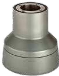
Swivel Base Internal Bracket Coupling for directly mounting enclosures to a machine or the floor. Turns through 340 degrees with rotation stop. Preset torque. Maintenance-free bearings. Type 304 polished stainless steel finish. Includes gaskets and enclosure mounting hardware. Base-mounting fasteners not provided.
