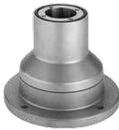
Swivel Base External Bracket Coupling for mounting enclosures directly to a machine or the floor. Turns through 340 degrees with rotation stop. Preset torque. Maintenance-free bearings. Type 304 polished stainless steel finish. Includes gaskets and enclosure mounting hardware. Base-mounting fasteners not provided.
