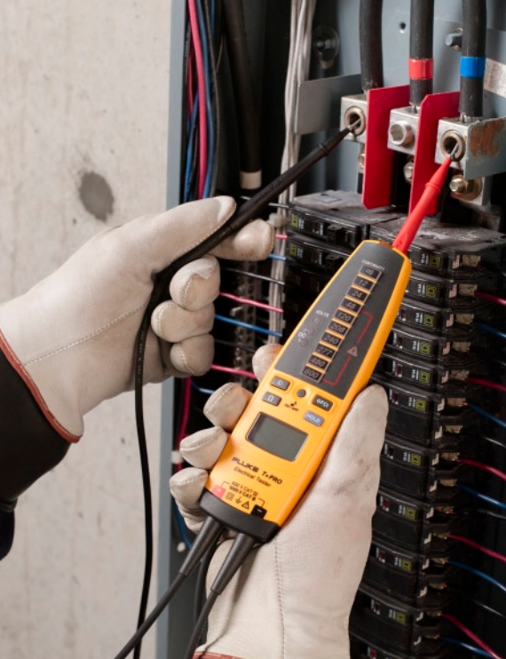
Electronic testers like this Fluke T+ vibrate, beep, and glow to indicate voltage, giving you the feel of an old-fashioned solenoid in a safer electronic model.
