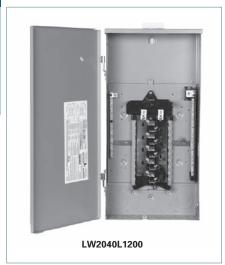
Load centers on this page through 225 amp feature a split neutral insulated bars. For service entrance applications, install bonding strap, and use both bars for neutral and ground conductors. For non service entrance applications, do not install bonding strap and use insulated bars for neutral conductors and bonded bar for ground conductors.
