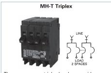
These space saver triplex breakers provide a 2-pole common trip breaker for 120/240V AC circuits and two single poles for 120V AC circuits. Triplex require two panel spaces. HACR rated.
