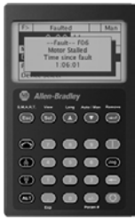
LCD Display, Full Numeric Keypad 20-HIM-A3
