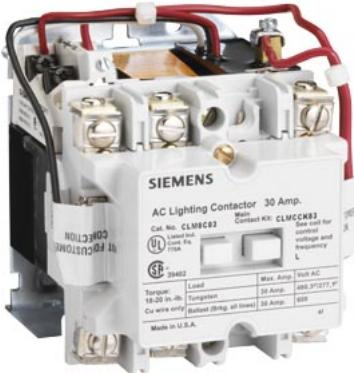
Mechanically held lighting contactor, Contactor amp rating 30A, 0 N.C. / 2 N.O. poles, 24VAC 60HZ coil, Non-combination type, Enclosure NEMA type (open), No enclosure
