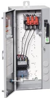
Non-reversing motor starter, Size 0, Three phase full voltage, Solid-state overload relay, OLR amp range 0.25-1A, 240V 50Hz / 277V 60Hz coil, Combination type, 30A non-fusible disconnect, Enclosure NEMA type 4/12, Water/dust tight for outdoors, Standard width enclosure
