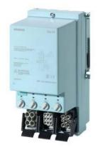
ET 200pro DSE HF DOL starter High Feature Mechanical switching Electronic overload protection AC-3, 0.9 kW / 400 V 0.15 A...2.00 A without brake contact 4 DI Han Q4/2 - Han Q8/0
