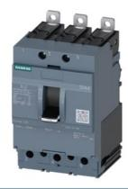
circuit breaker 3VA4 UL Frame 125 breaking capacity class H 65 kA @ 480 V 3-pole, line protection TM210, FTFM, In=30 A overload protection Ir=30 A permanently set short-circuit protection Ii=10 x In terminal connection
