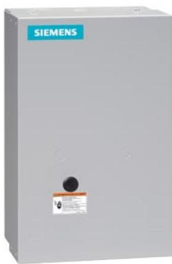
Mechanically held lighting contactor, Contactor amp rating 100A, 0 N.C. / 3 N.O. poles, 220VAC 50HZ/240VAC 60HZ coil, Non-combination type, Enclosure NEMA type 1, Indoor general purpose use
