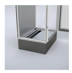
**Description:** Suspended below the bottom plates, thereby maximizing the full usable space in the enclosure. Holds standard cable clamps CAC to secure incoming cables. Fully adjustable in depth. When EMC shielded earthing cables are connected to the support bar the Faraday effect will be kept intact for maximum EMI shielding.
