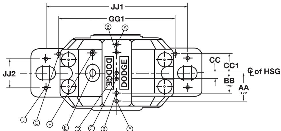
**Figure 3 Dowel Pin Locations**
