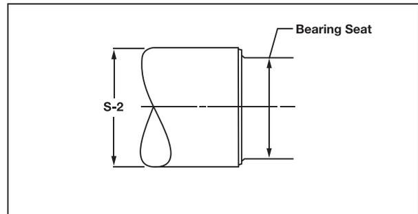
**Figure 2 - Shaft Diameter**
