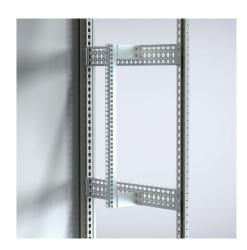
**Description:** Partial height 19" vertical profiles to achieve 482.6 mm (19") mounting requirements on all sides. Adjustable in depth in steps of 25 mm using the CLPK click-in profiles.
