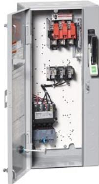
Non-reversing motor starter, Size 0, Three phase full voltage, Solid-state overload relay, OLR amp range 5.5-22A, 110V 50Hz / 120V 60Hz coil, Combination type, 30A fusible disconnect, 30A/250V fuse clip, Enclosure NEMA type 1, Indoor general purpose use, Standard width enclosure
