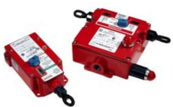
CPS Series Cable Pull Safety Switches provide a readily accessible emergency stop signal. This is a cost-effective means compared to using multiple emergency stop push-buttons. (Cable Pull Safety Switches are not, however, to be used as a means of personnel safeguarding. They may be used to prevent further injury or damage to equipment when used for emergency stop signaling.)
