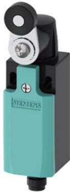
Position switch Plastic enclosure according to EN 50047, 31 mm 1 NO/1 NC quick action contacts integrated (not replaceable) with M12 connector, 4-pole Pin assignment: Pin1=21, Pin2=22 Pin3=13, Pin4=14 for max. 250 V and 4 A Twist lever, right and/or left switching can be set with plastic roller 19 mm
