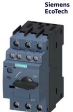
Circuit breaker size S00 for motor protection, CLASS 10 A-release 5.5...8 A N-release 104 A screw terminal Standard switching capacity with transverse auxiliary switches 1 NO+1 NC
