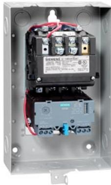
Non-reversing motor starter, Size 1, Three phase full voltage, Solid-state overload relay, OLR amp range 10-40A, Non-combination type, Enclosure type 1, Indoor general purpose use, Standard width enclosure
