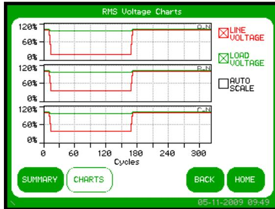
Line voltage is shown in red and load voltage is shown in green. By pressing the check boxes in the right column, you can toggle each data series Off and On as well as enable y-axis auto-scaling.
