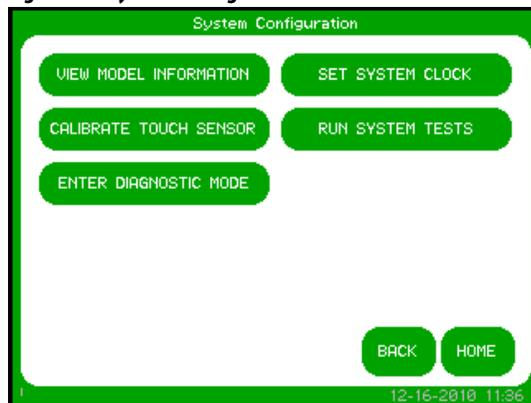
**IMPORTANT** To recalibrate from any screen, hold anywhere on the screen for 10 seconds. You will see a small progress bar at the bottom of the screen. When the progress bar reaches 100 percent, the calibration screen will open.
