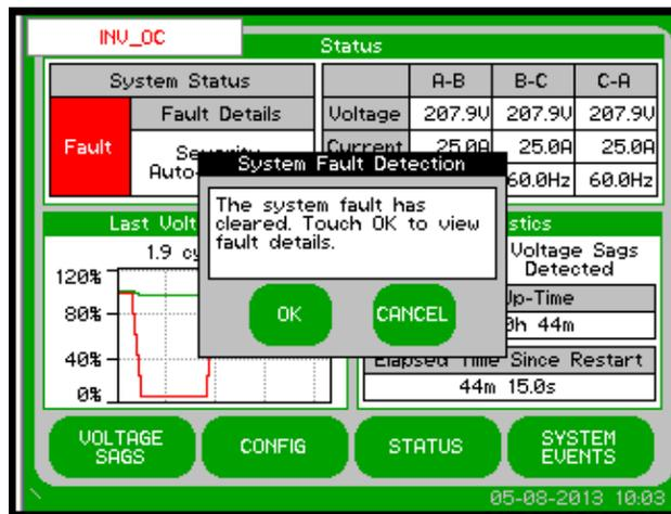
If a “Call Service” severity event is detected, record the event details including: name, description, location, and reading. Contact product support immediately. If the event clears, the touch screen will automatically go back to normal operation.
