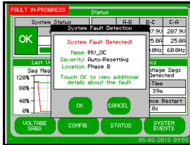
Pressing the “OK” button will open the “System Event Detail” screen. The event will appear in the event list after the event is over. The window can be closed by pressing the “CANCEL” button or waiting 15 seconds.
