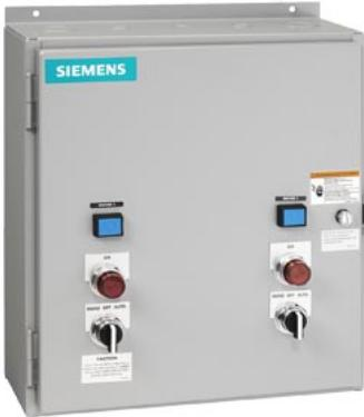
Duplex starter w/ alternator, Size 2 1/2, Three phase full voltage, Solid-state overload relay, OLR amp range 25-100A, 110V 50Hz / 120V 60Hz coil, Non-combination type, Enclosure NEMA type 1, Indoor general purpose use
