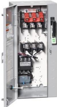
Non-reversing motor starter, Size 2, Three phase full voltage, Solid-state overload relay, OLR amp range 13-52A, 110V 50Hz / 120V 60Hz coil, Combination type, 60A fusible disconnect, 60A/250V fuse clip, Enclosure NEMA type 1, Indoor general purpose use, Standard width enclosure
