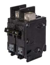
Siemens Low Voltage Molded Case Circuit Breakers General Purpose MCCBs - Type BQ, 2-Pole, 120/240VAC are Circuit Protection Molded Case Circuit Breakers. 2-Pole Common-Trip circuit breaker type BQ. Rated 120/240V (045A) (AIR 10 kA). Special features: line side lugs included. Note: Load side lugs are included.
