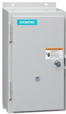
Non-reversing motor starter, Size 2 1/2, Three phase full voltage, Solid-state overload relay, OLR amp range 25-100A, 110V 50Hz / 120V 60Hz coil, Non-combination type, Enclosure type 12, Dust/drip proof for indoors, Standard width enclosure
