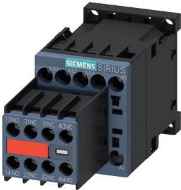
power contactor, AC-3e/AC-3, 9 A, 4 kW / 400 V, 3-pole, 110 V AC, 50 Hz / 120 V, 60 Hz, auxiliary contacts: 2 NO + 2 NC, screw terminal, size: S00, captive auxiliary switch
