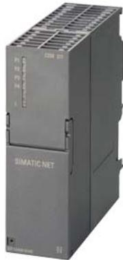
Compact Switch Module CSM 377 Connection SIMATIC S7-300 and up to 3 further nodes to Industrial Ethernet with 10/100 Mbit/s unmanaged switch, 4 RJ45 ports, External 24 V DC power supply LED diagnostics, S7-300 module, incl. electron. Equipment Manual on CD-ROM.
