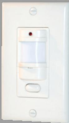
Fits decorator wall plates with only 1/2" protrusion. Gangable. Sensitive 180° view passive infrared motion detector keeps lights on only when rooms are in use covers 1000 sq. ft. Works with electronic ballasts. Can be wired in parallel. LED indicator, wallplate included. Can also be used as a ceiling sensor. Must have hot and wires in box.
