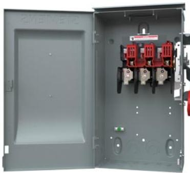
Siemens Low Voltage Circuit Protection Heavy Duty Safety Switch. 3-Pole 3-Wire and negative ground Non-Fused in a type 3R enclosure (outdoor). Rated 600VAC (30A). Special features: photovoltaic rated, 10000 AIC disconnect.
