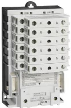
Electrically held lighting contactor, (convertible to mech. held), Amp rating 30A (tungsten 20A), 0 N.C. / 6 N.O. poles, 277V 60Hz / 240V 50Hz coil, Non-combination type, Enclosure NEMA type (open), No enclosure
