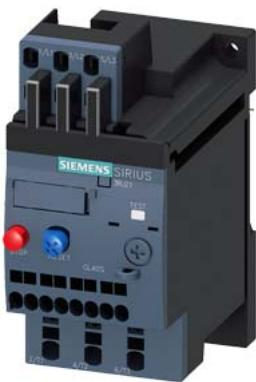
Overload relay 11...16 A Thermal For motor protection Size S00, Class 10 Stand-alone installation Main circuit: Spring-type terminal Auxiliary circuit: spring-type terminal Manual-Automatic-Reset
