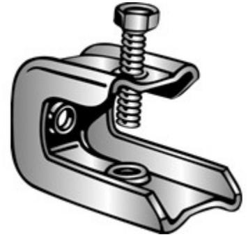
*Set Screw Beam Clamp, Fits Up to 3/4" Flange, 3/8"-16 Tapped Holes Bottom and Back of Beam Clamp, Type 304 Stainless Steel*
