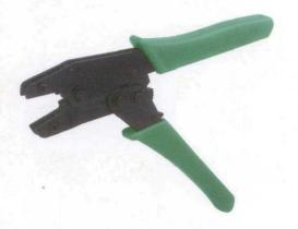
The KWIK CYCLE® 8 features a smaller handle spread with a comfortable, ergonomically designed handle. This tool frame is very popular for the higher production environment and for the hard to handle smaller connectors such as fiber optic connectors and open barrel contacts. All KWIK CYCLE® 8 crimping die sets are easily interchangeable with a simple screwdriver.
