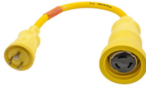
Adapter, Marine, Molded, Straight Blade, 30A 125V 2-Pole 3-Wire Grounding Female to 50A 125V, 2-Pole 3-Wire Grounding Locking Male
