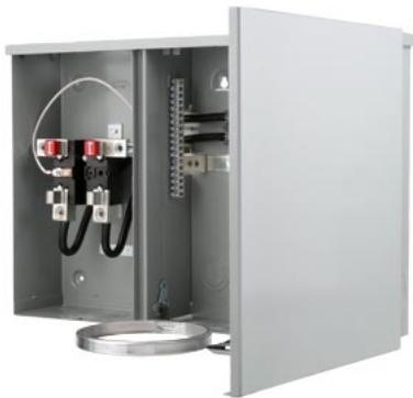
SIEMENS LOW VOLTAGE METER LOAD CENTER COMBINATION. FACTORY INSTALLED MAIN BREAKER 12 (1 INCH) SPACES INTERIOR ALLOWING MAX 24 CIRCUITS. 4-JAW METER / 1-PHASE SYSTEM RATED 125A. SPECIAL FEATURES: OH/UG FEED RING TYPE COVER
