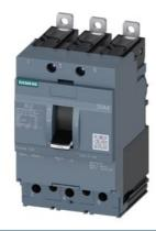
circuit breaker 3VA4 UL Frame 125 breaking capacity class S 25 kA @ 480 V 3-pole, line protection TM210, FTFM, In=30 A overload protection Ir=30 A permanently set short-circuit protection Ii=10 x In UL489 SB (naval), 50 degrees Celsius terminal connection
