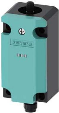
Basic switch for position switch 3SE51 Metal enclosure 40 mm according to EN 50041 1 NO/1 NC quick action contacts with M12 connector, 5-pole, fixed with 2 LEDs, yellow/green, 24 V DC without actuator head Pin assignment: Pin1=21, Pin2=22 Pin3=13 and LED green, Pin4=14 and LED yellow, Pin5=ground LED
