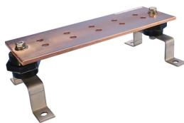
Proper bonding is essential to create an equipotential plane between service grounds and equipment during fault and transient conditions. This equipotential plane provides a near-zero voltage differential, and serves to protect people and equipment during these events. The grounding busbar is the most popular bonding product in use today.
