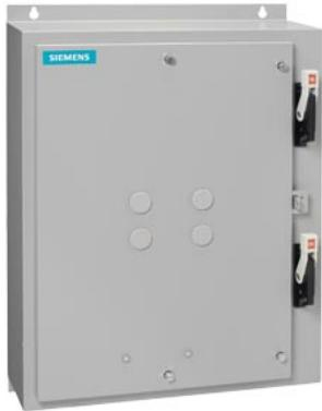
Duplex starter w/ alternator, Size 2 1/2, Three phase full voltage, Solid-state overload relay, OLR amp range 25-100A, 110V 50Hz / 120V 60Hz coil, Combination type, Two 100A circuit breakers, Enclosure NEMA type 12, Dust/drip proof for indoors
