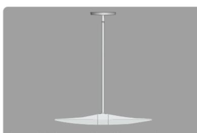
The PLED is a high performance LED uplight available in 52, 40, 26 and 20W versions in both Cool and Warm Color Temperatures. Pendant mount with hang-straight and 6", 12" and 18" stems included. Stems can be combined up to 36" max length.
