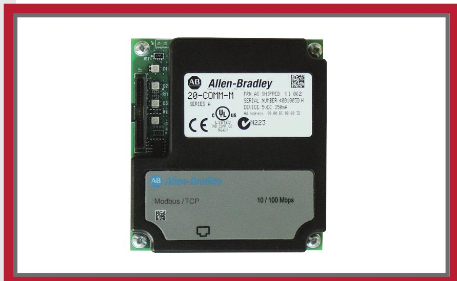
**Supported Modbus Function Codes** – Unlike most drive communication adapters, Modbus/TCP adapters use Function Codes to view logic status, feedback and parameter values, send logic control, reference, and change parameter values. The following Function Codes are supported by the adapter:
