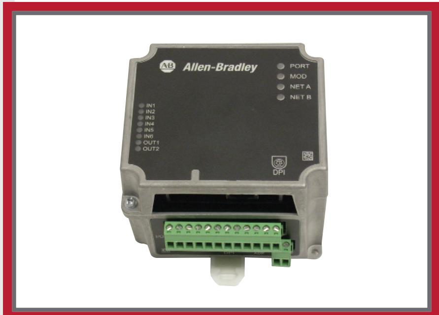
installed in the kit for applications that require additional general-purpose network I/O that a controller can use. The drive and I/O devices are handled as one node on the network, saving network node count and increasing network throughput.
