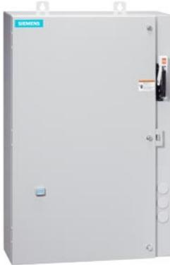
Non-reversing motor starter, Size 2, Three phase full voltage, Solid-state overload relay, OLR amp range 13-52A, Combination type, 50A circuit breaker, Enclosure NEMA type 4/12, Water/dust tight for outdoors, Extra-wide enclosure
