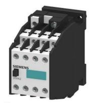
Contactor relay, 62E, DIN EN 50011, 6 NO 2 NC, screw terminal AC operation 24 AC 50/60 Hz
