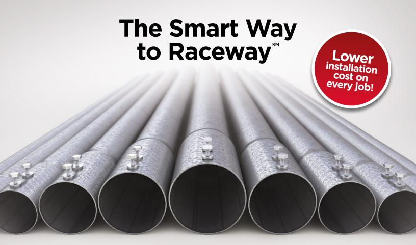
With SmartSet, you don't have to purchase, inventory and install separate couplings. The engineered steel set screw coupling comes built into one end of every piece of EMT so you can work smarter—saving you time and money on every job. SmartSet EMT is available in trade sizes 1½-4 and in 10' and 20' lengths.
