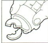
Split slugs fall free from the die and stud.
